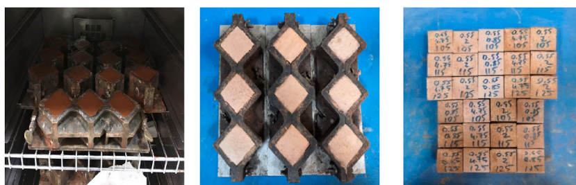
Fig. 5. Views of cubic specimens in the fresh state, after curing, and in the hardened state (left to right).
