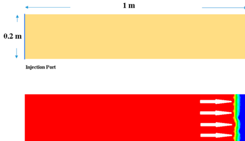
Figure 3. Analyzed case of unidirectional injection in a rectangular mold cavity: the flow advances from the left side (injection port) toward the right side (vent).
