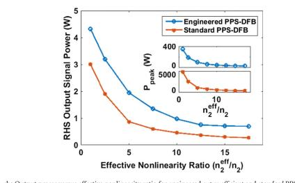
Figure 6. rhs Output power versus effective nonlinearity ratio for engineered *super-efficient* and *standard* PPS-DFB. The inset shows the intra-cavity peak power versus effective nonlinearity ratio.
