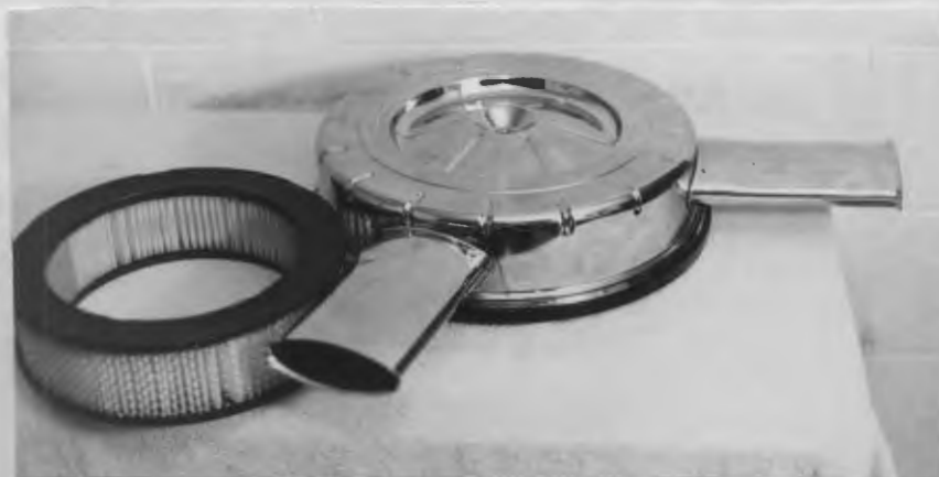
Figure 10. General Motors Dual Snorkel Air Cleaner Housing
