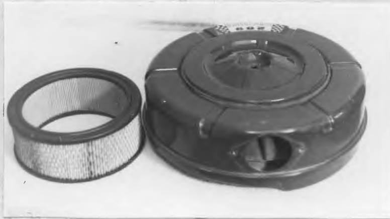
Figure 2. Factory Equipment Air Cleaner Without Snorkel
