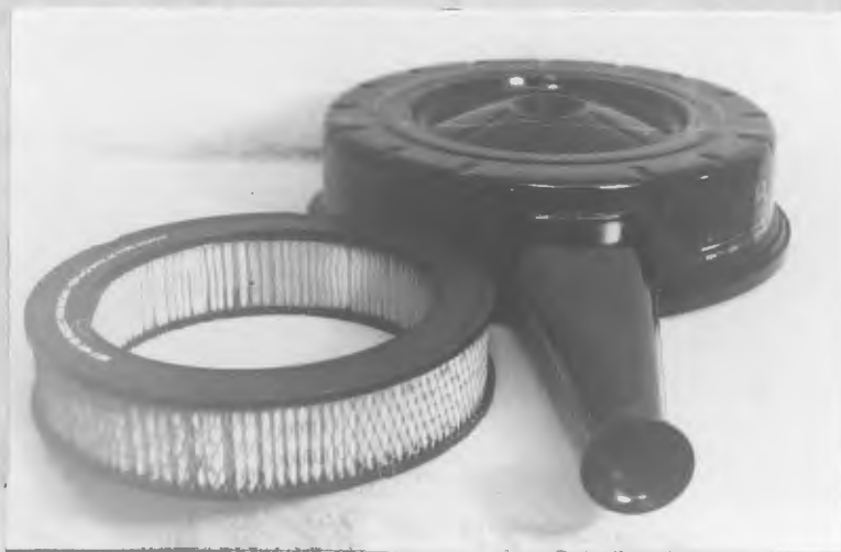
Figure 13. General Motors Air Cleaner Housing With Small Filter Element
