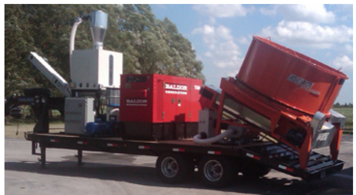
Image 4.2 Buskirk Engineering's Mobile Pelletizing Unit, image retrieved from Buskirk Engineering's website.
