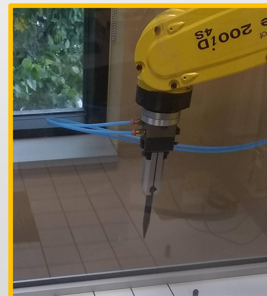
FANUC LR Mate 200iD 4s end of arm tooling holding a graphite stick
