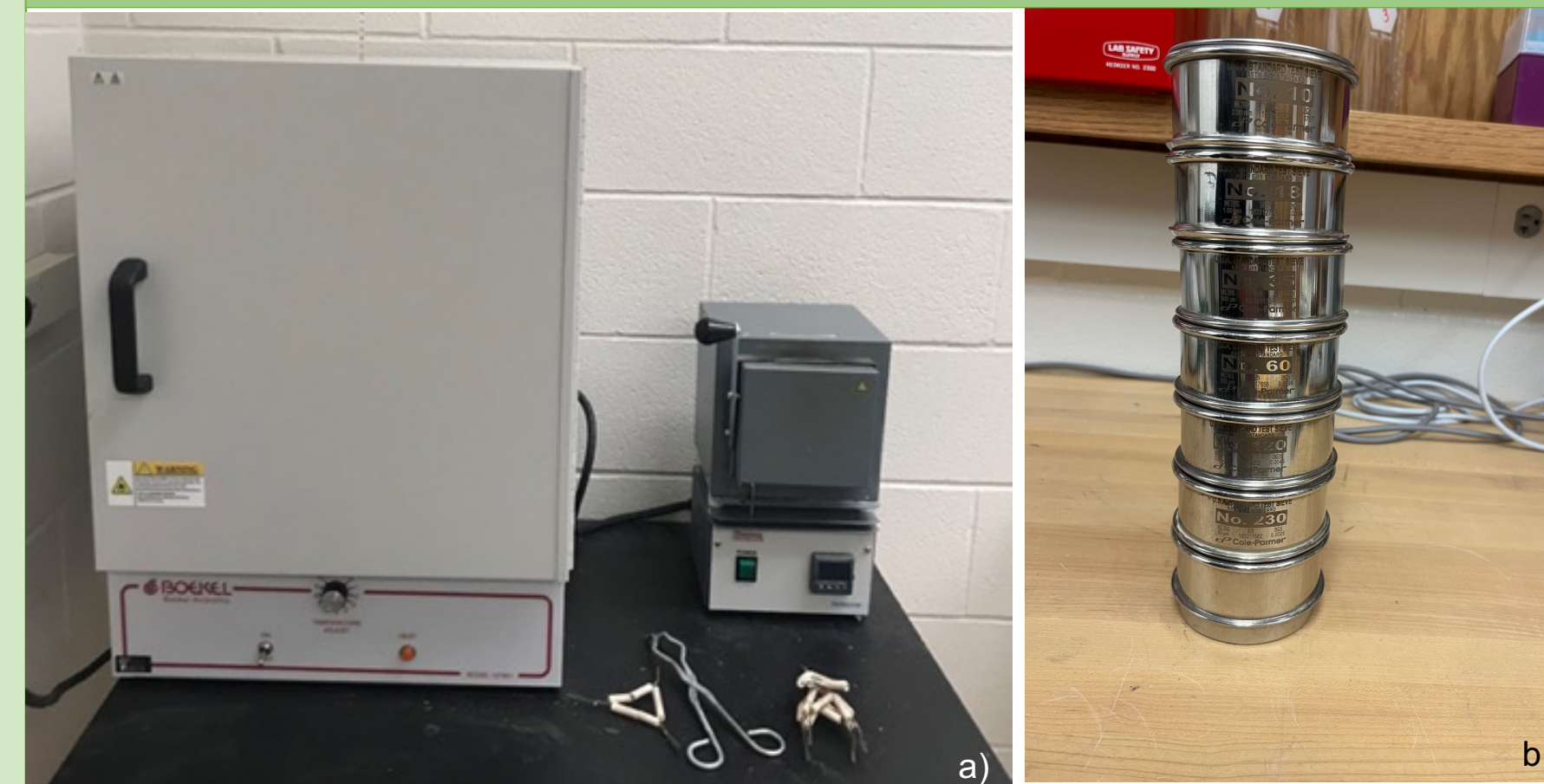
a) The drying oven that was used to remove water from the samples (Left). The Muffle Furnace used to remove the organics from the samples (Right). b) The set of sieves used to separate the grains for the grain size analysis.
