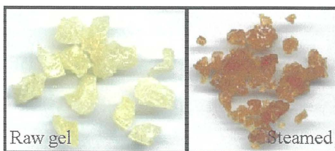
Figure 5.1.3: Photographs showing the appearance of gels prior to and after steam treatment.
