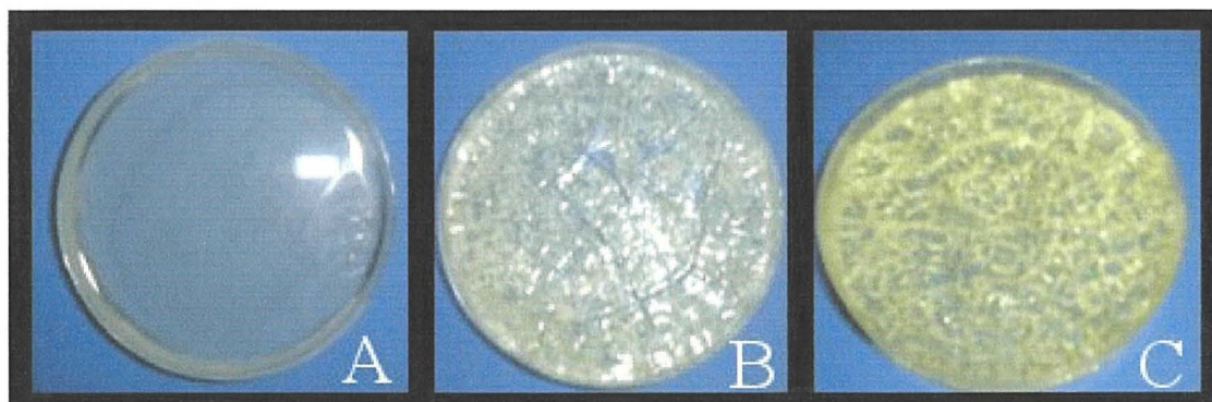
Figure 3.1.7: Bulk gels in the covered raw state, A, the uncovered raw state, B and the final aged state, C showing changes in colour and texture.
