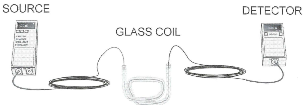
Figure 2.1.9: Apparatus used to test the response of sensors that were fully immersed in analyte liquids. A handheld light source and power meter were connected to either end of a sensor cable. A 1 m length of sensor was contained in a glass coil which was filled with the liquid under test.
