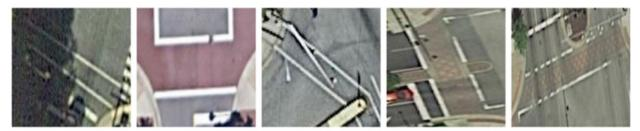
(c) Correctly classified crosswalks (Ground truth: High, High, High, Low, Low; Predict: High, High, High, Low, Low)
