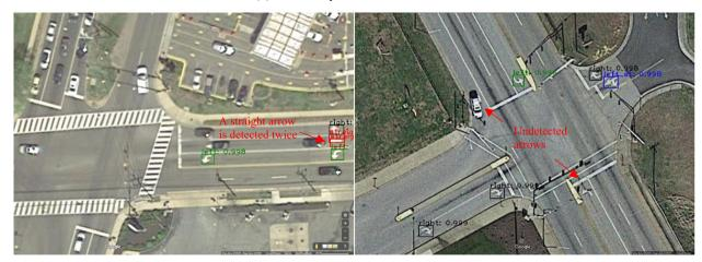
(b) Incorrectly detected lane-use arrows Fig. 12 Example of correctly detected and incorrectly detected lane-use arrows (Numbers indicate confidence levels)
