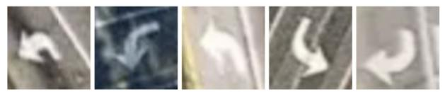
(b) Incorrectly classified lane-use arrows (Ground truth: High, High, High, Low, Low; Predict: Low, Low, Low, High, High)
