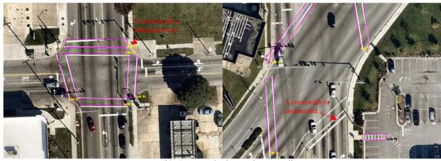
(b) Incorrectly detected crosswalks Fig. 13 Examples of correctly detected and incorrectly detected crosswalks (Numbers indicate confidence levels)
