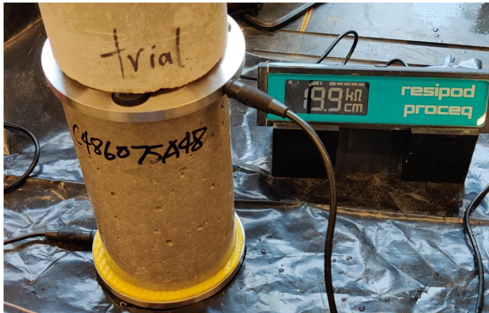
Figure 13. Bulk electrical resistivity test set-up.
