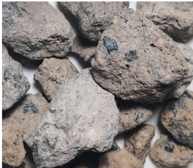
Figure 2. Pieces of recycled concrete aggregates.
