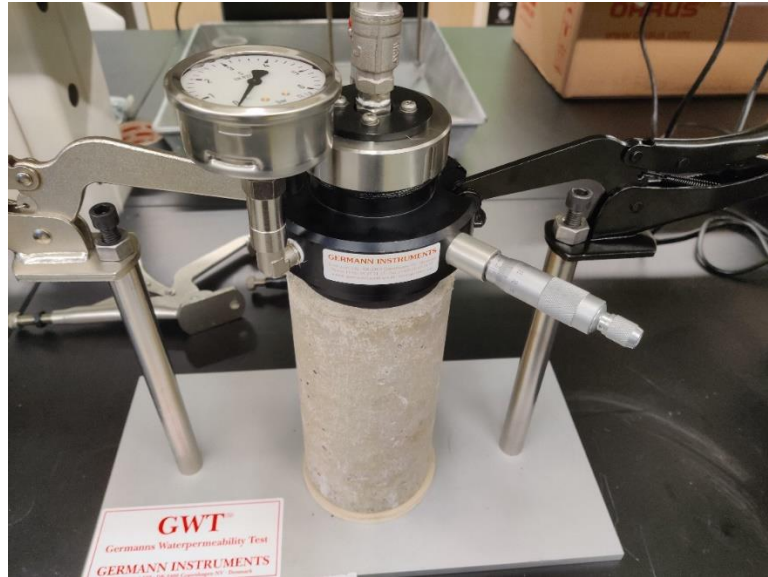
Figure 14. Germann Water Permeability Test (GWT) set-up.
