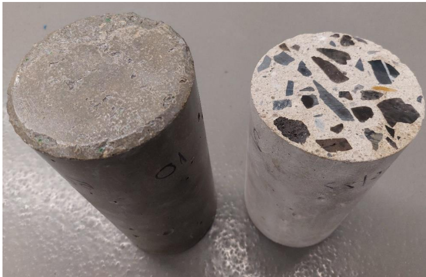
Figure 10. Concrete specimens (left) before and (right) after cutting the surface.
