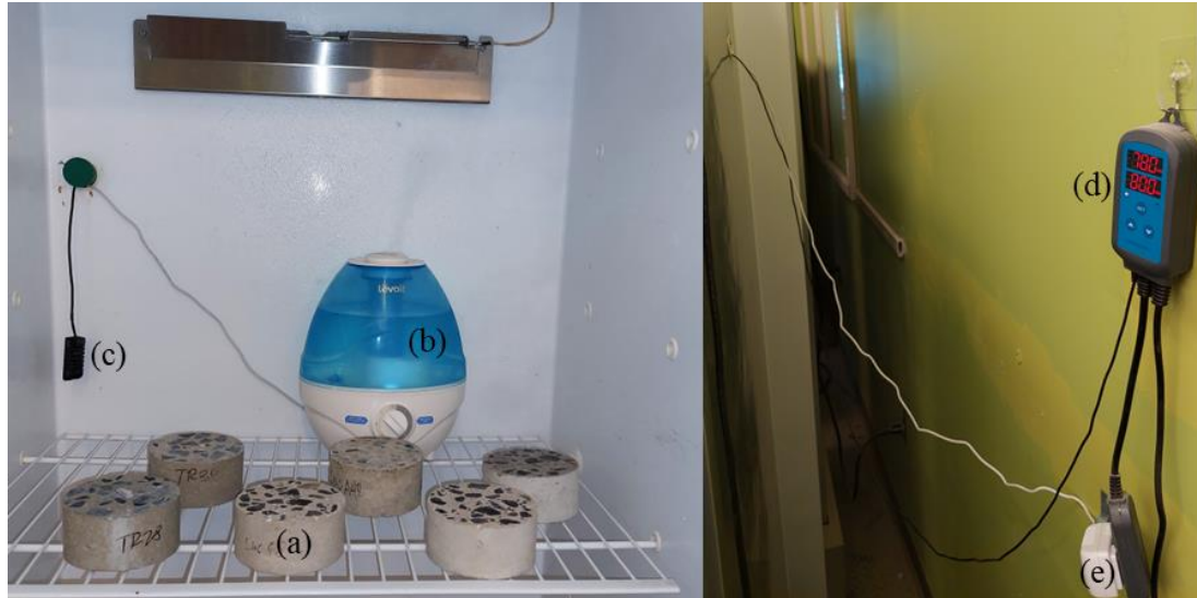
Figure 16. Sorptivity conditioning set-up showing (a) concrete specimens, (b) mist humidifier, (c) humidity sensor inside the environmental chamber, (d) humidity controller, and (e) humidifier power plug.
