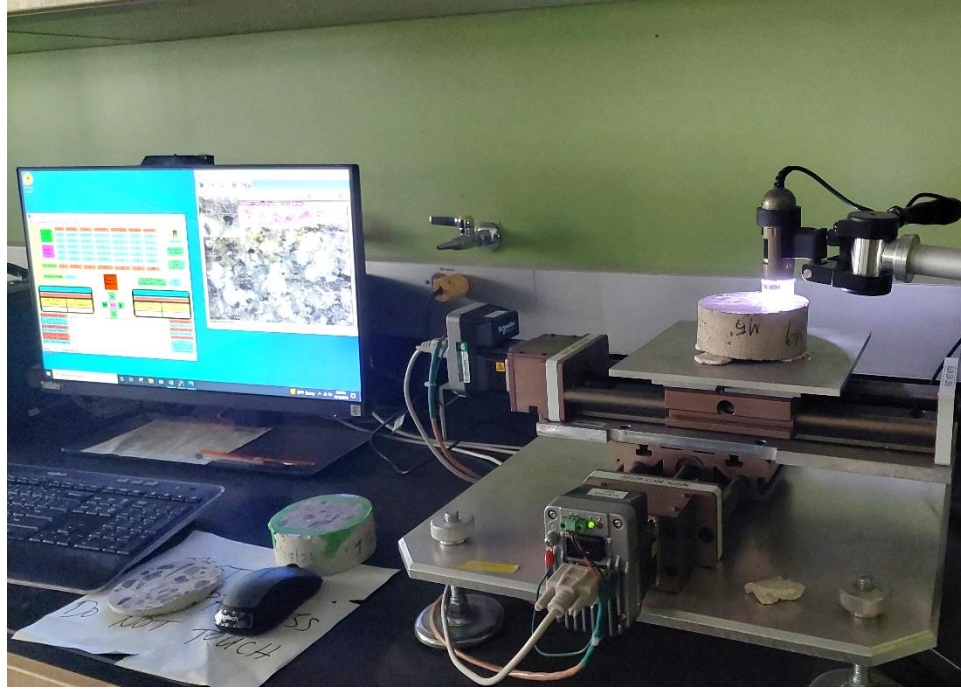
Figure 21. Linear traverse machine set-up.
