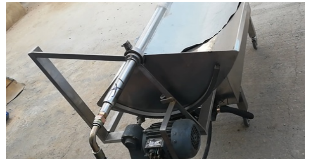
Figure 6. AC Motor and Track Used in the Single-Axis Tracking System
