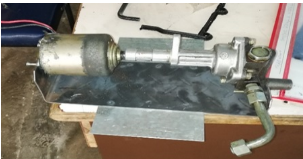
Figure 4. The 12V DC Hydraulic Pump Used in PTC
