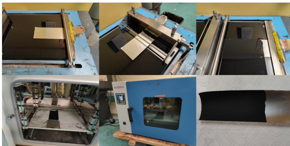
Figure 3.3.5: Doctor blading the coating and drying
