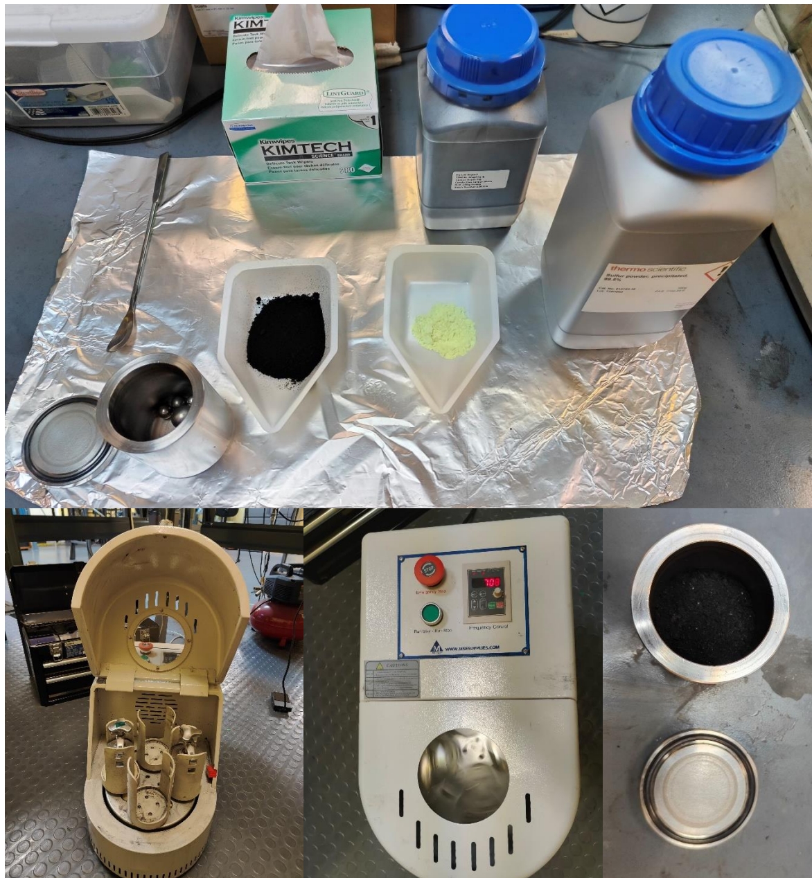
Figure 3.3.1: Ball milling setup used in the cathode coating process.
