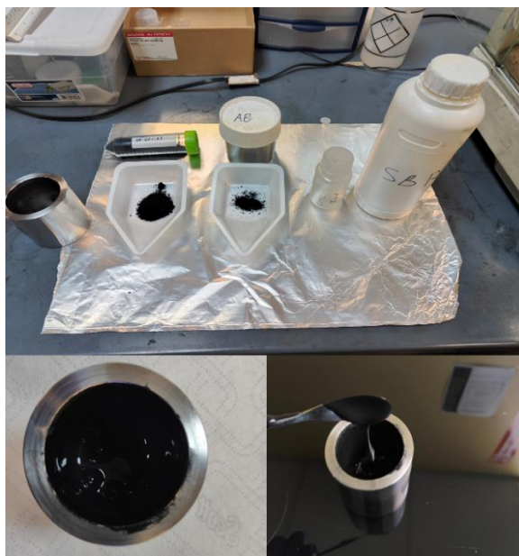
Figure 3.3.4: Slurry mixture and its texture before coating
