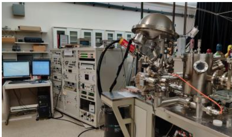
Figure 2.6.2.1: VG Scientific MultiLab 3000 XPS system
