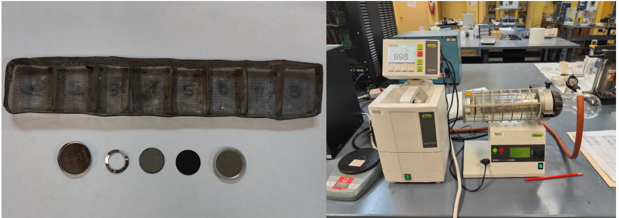
Figure 3.4.1: Drying cathodes, coin cell cases and current collectors.
