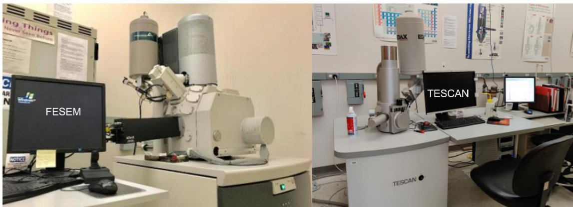
Figure 2.6.1.2: FESEM and TESCAN SEM systems
