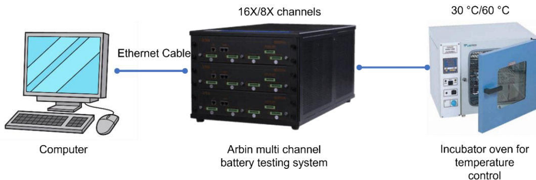
Figure 2.7.3.1: Battery testing system with temperature control used for this work,
