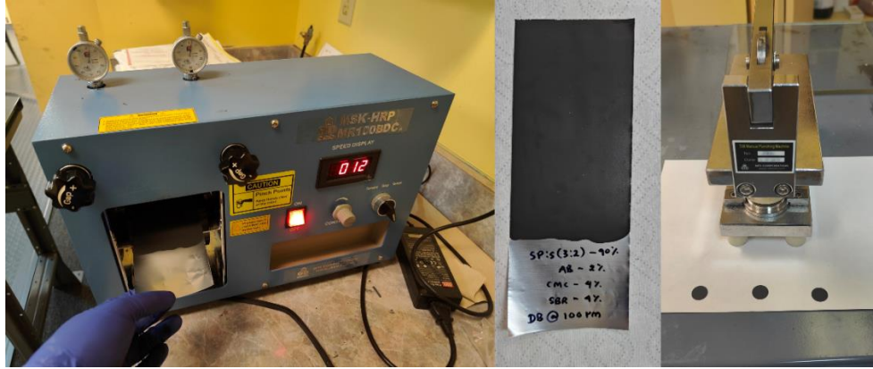
Figure 3.3.6: Calendaring and electrode punching
