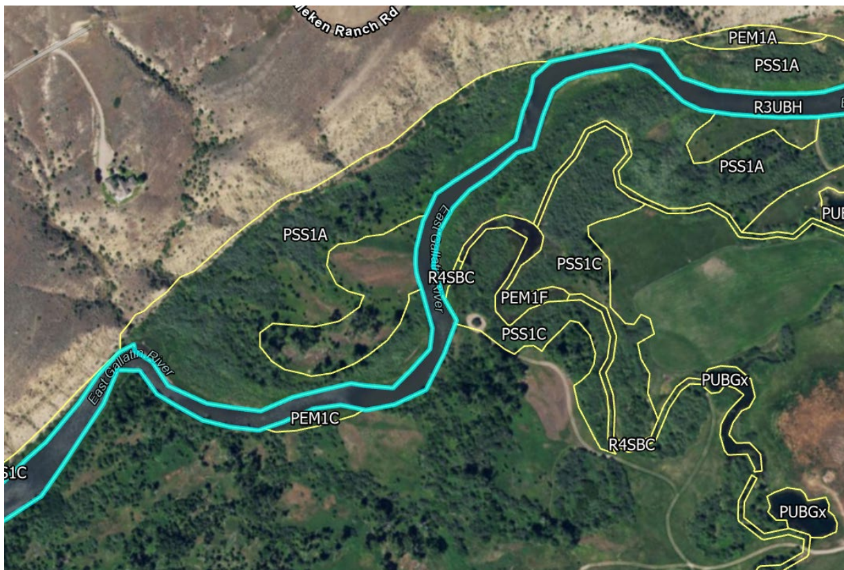
Figure 3. Classification of Upper-perennial Riverine (R3), Intermittent stream (R4), Palustrine Emergent (PEM), Palustrine Scrub-Shrub (PSS), and Palustrine Unconsolidated Bottom (PUB) near the East Gallatin River in the Nixon Gulch quad. The NAIP basemap imagery shown is at 1:4,505 scale.
