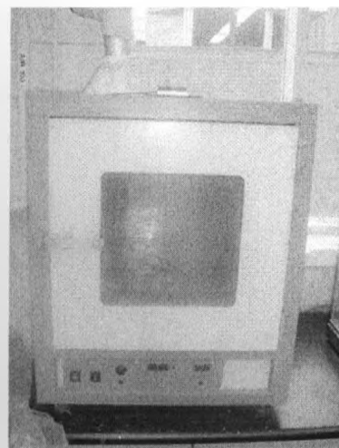
Figure 7.12: Convection oven for curing
