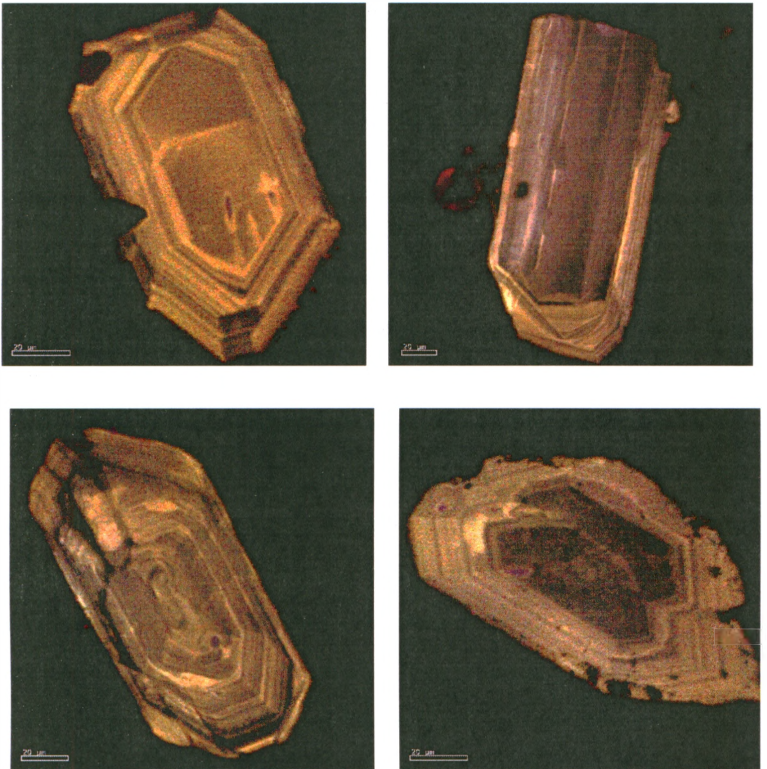
Figure 3.19. Representative CL patterns of zircons from the Bighorn River Bentonite. All show oscillatory zoning, and some show sector zoning (Bottom left image). The bottom right zircon shows a composite zircon CL image, where two grains were sutured together.
