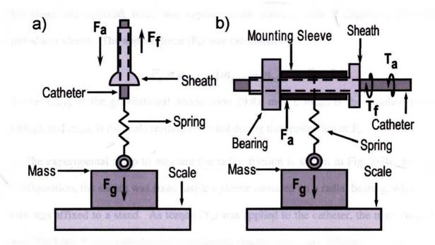
Fig. 2-2: Experimental setup to measure resistive force caused by introducer sheath in a) axial direction (vertical stand not shown), and b) radial direction.
