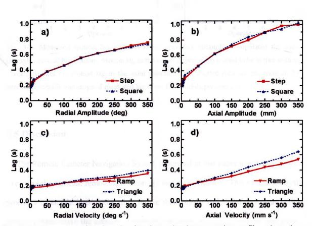
Fig. 3-4: Measured replicated motion lag time using known motion profiles: a) step/square response in the radial direction, b) step/square response in the axial direction, c) ramp/triangle response in the radial direction, and d) ramp/triangle response in the axial direction.
