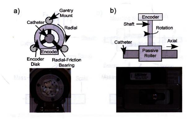
Fig. 2-1: Motion sensing device: a) catheter rotation is measured by rotating the optical encoder disk via 3 radial-friction bearings, and b) axial motion is measured as the catheter moves against a passive roller, which rotates the disk of a second optical encoder. Below each schematic is a photograph of the corresponding manufactured sensor.
