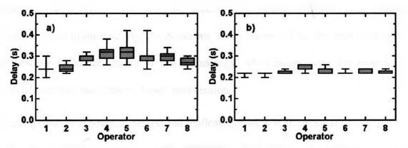
Fig. 3-5: Measured motion lag when different operators remotely manipulated the catheter through a carotid bifurcation. Motion lag in the radial direction (a) tended to be higher with more variability than the motion lag in the axial direction (b). Plotted data are the median, 25-75 percent percentile and range of measured lag times for 12 trials per operator.
