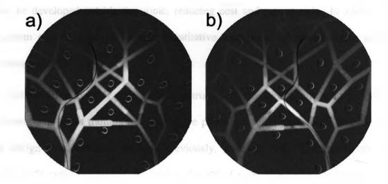
Fig. D-3: Radiographs of the multi-path training phantom injected with contrast via the left inlet (a), and right inlet (b). The catheter is clearly visible in both images.
