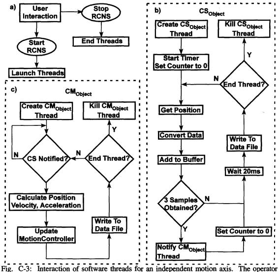
rig. C-3: interaction of software threads for an independent motion axis. The operator enables tele-operated catheter navigation (a), creating four software threads, one for each peripheral device axis, which run independent of the main program. A thread corresponding the CS axis, samples the CS at 20 ms intervals, after three samples the thread notifies the corresponding CM thread.
