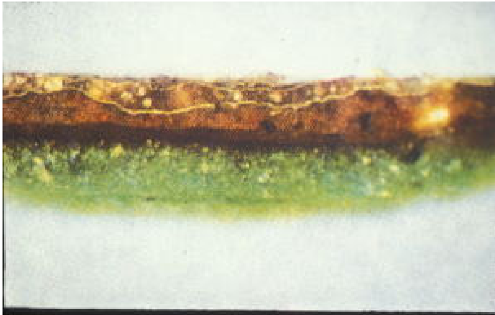
11. Microscopic cross-section of vertical inscription of left wing (140x), layers from lower to upper: green, yellow-brown glaze, yellow-brown binding medium, original twist gold (silver/gold), binding medium of second application, gold leaf of second application, binding medium of new restoration, gold leaf of new restoration, St. Magdalene Altarpiece .
