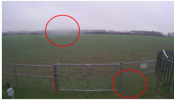
Figure 3.6: Image from the Batavia station with moisture build up on the lens circled in red.
