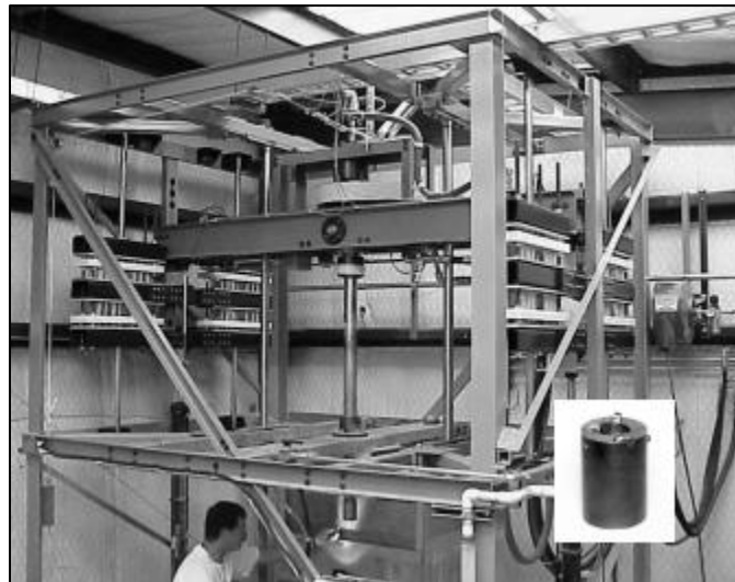
Figure 2.5. SNL Mechanical Analog Drillstring (Raymond et al., 2008)
