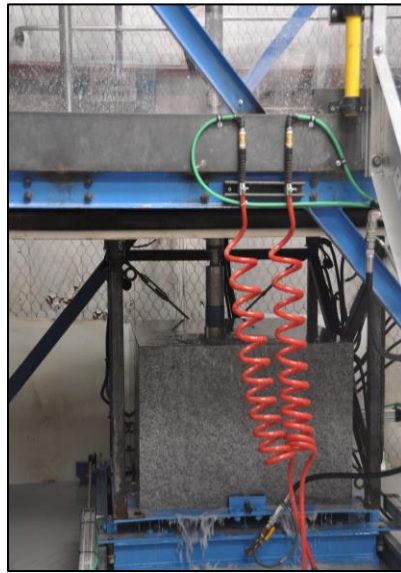
Figure 3.2. HRDF Platform with Rock Sample (Barnett et al., 2022)
