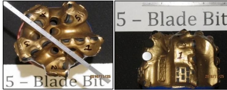
Figure 3.5. Profile of the 5-Bladed PDC Bit (Barnett et al., 2022)
