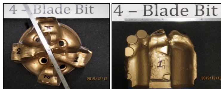
Figure 3.4 Profile of the 4-Bladed PDC Bit (Barnett et al., 2022)
