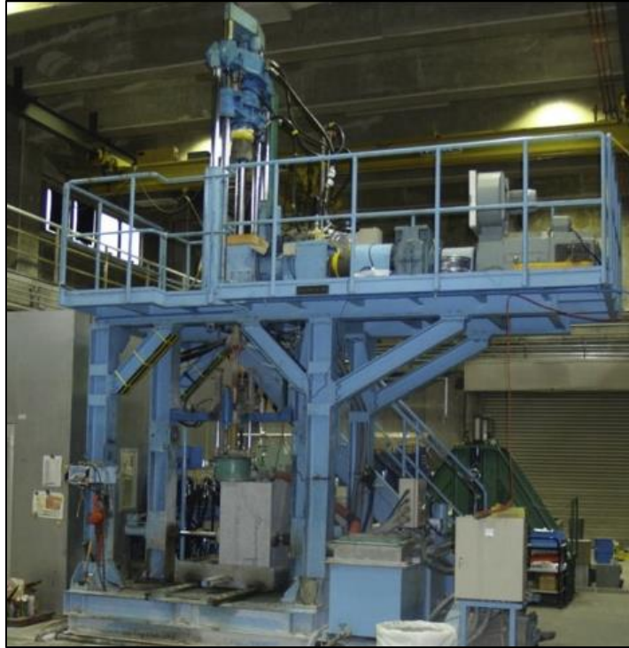
Figure 2.2. Laboratory Drillstring Overview (Miyazaki et al., 2019)
