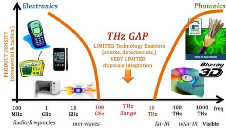
Figure 1.1. Representation of the THz region in the EM spectrum [1]
