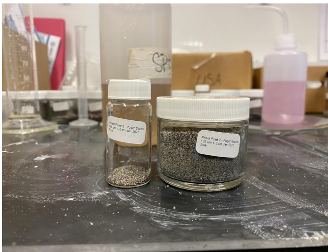
Figure 5: The difference in size between the float sediments (left) and the sink sediments (right) of the 125 \mu\text{m} from Priest Point 2.
