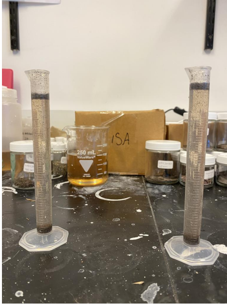
Figure 4: The separation of West Bay sediments using the SPT method
