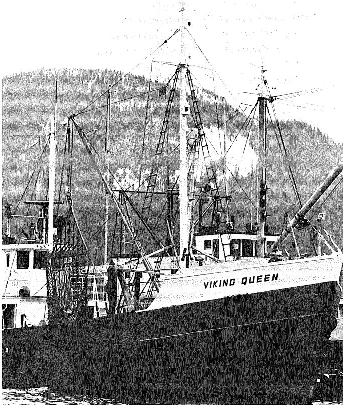
THE "VIKING QUEEN," 90-FOOT NEW BEDFORD SCALLOPER, CHARTERED BY THE STATE OF ALASKA FOR SURVEY OF ALASKA SCALLOP RESOURCES —BCF Photo
