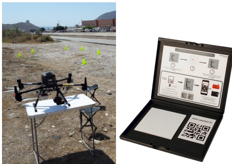
Figure 17. Micasense dual camera system used for data collection. Left: DJI Matrice 210 V2 equipped with Micasense dual sensor. Right: Micasense reflecting panel (Micasense, 2022)
