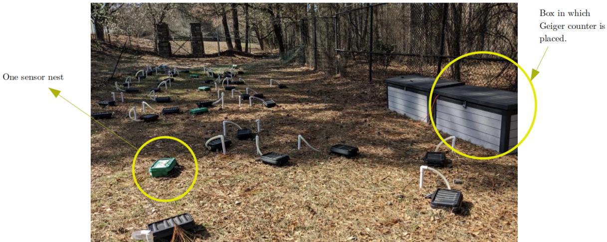
Figure 3.1: Radon testbed at Stone Mountain, GA, USA.
