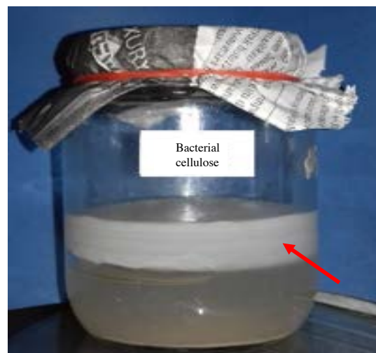
Fig. 1: Formation of bacterial cellulose (BC) pellicle on the surface of sago liquid waste medium after 14th days fermentation The arrow showed the BC pellicle
