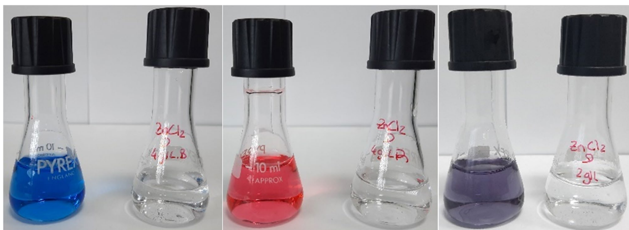
Fig. 8 Effect on color intensity with the maximum dose of adsorbent on dye removal (pH = 2; initial dye concentration: 25 mg L -1 ; adsorbent dose: 4 g L -1 for blue and red dyes and 2 g L -1 for black; contact
