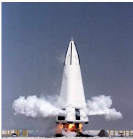
Figure 2.1: NASA picture of the DC-XA (1996): unsuccessful project for a prototype SSTO reusable vehicle with the main goal of performing a vertical take-off and landing.
