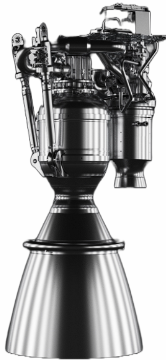
Figure 2.6: Sea-Level Merlin engine used on Falcon 9 and Falcon Heavy first stages.
