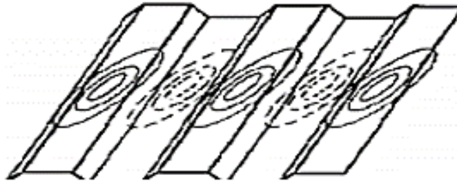
Figure 1.21. Interactive buckling mode of corrugated plates.
