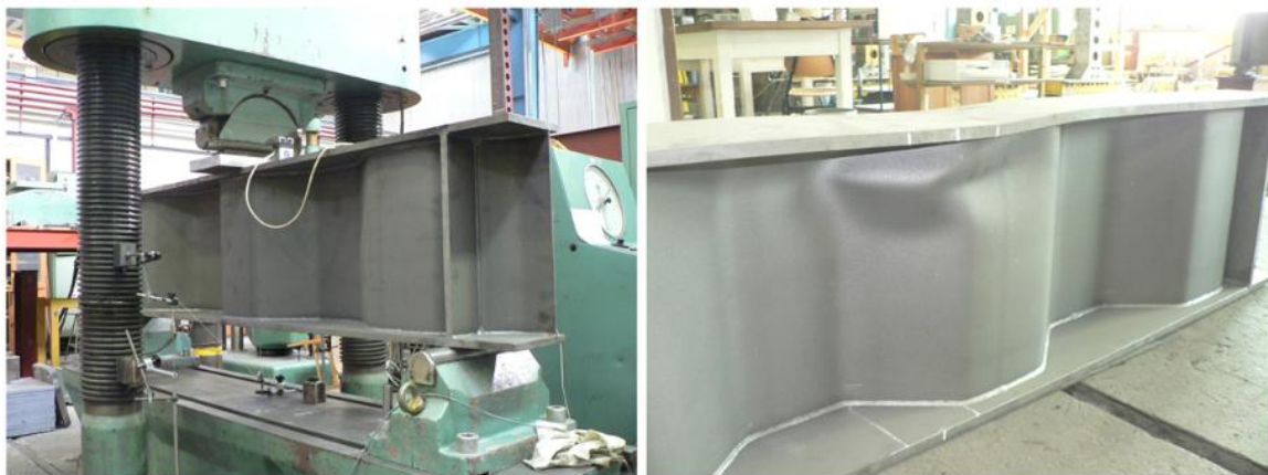
Figure 1.23. Test specimen arrangement and typical failure mode
