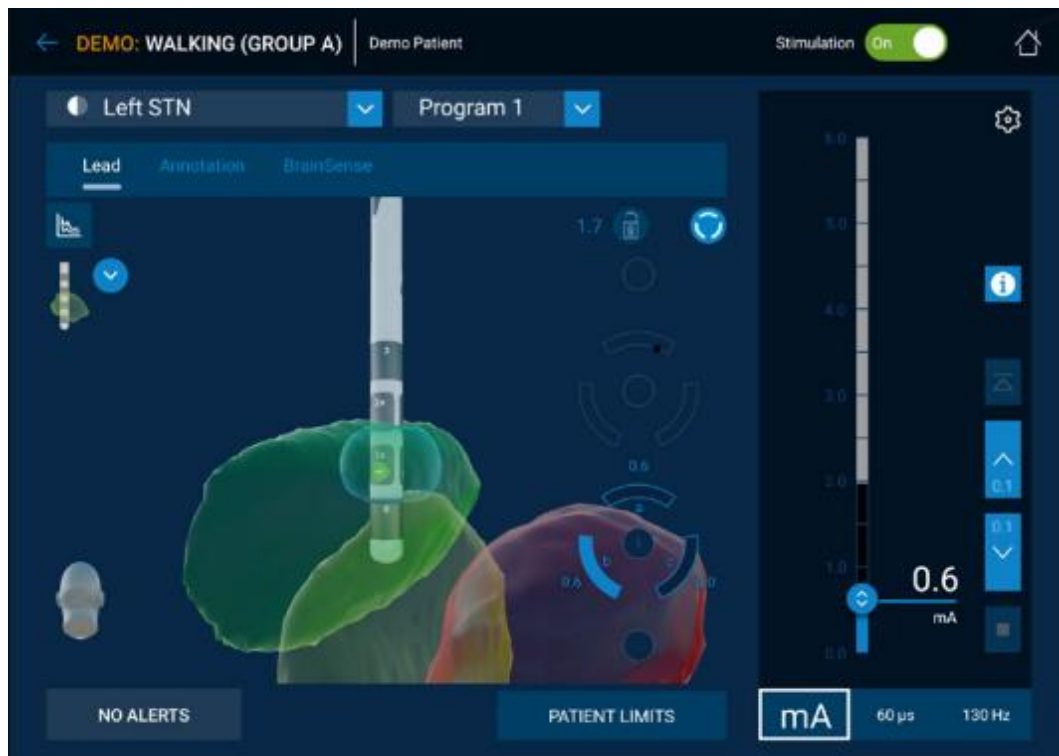
Figure 18: Example of the clinical interface used by Medtronic to display the anatomical context of the DBS lead.
