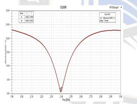
Fig. 3. VSWR versus frequency plot of the patch antenna
