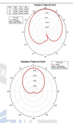
Fig. 4. 2D Radiation pattern; (a) E field radiation pattern, (b) H field radiation pattern
