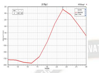
Fig. 6. Gain versus frequency plot of the patch antenna
