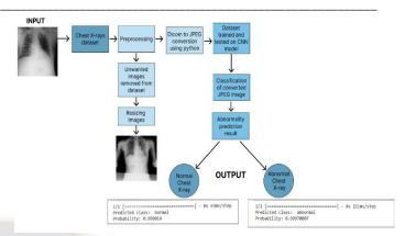
Figure 1. step-by-step classification and conversion process of CNN model.
