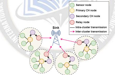
Figure 2. WSN Architecture using WMCL-DLRS-CRP
