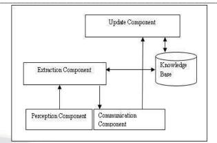
Figure 3.Architecture of Boundary Interface Agent
