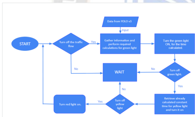
Figure 3 - Traffic light switching flow chart
