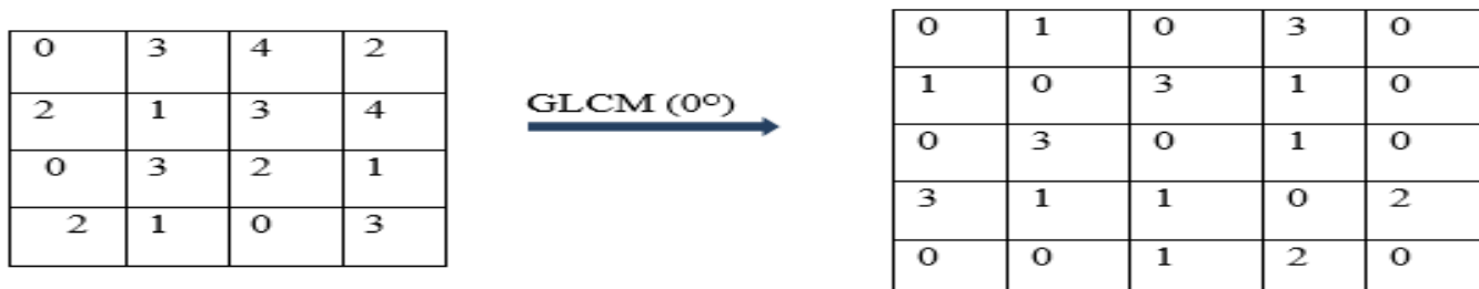
Figure 7. A) Grey Levels Of Mammogram Image B) Co-Occurrence Matrix Obtained By 0° From Grey Levels Of Mammogram Image
