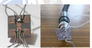
Figure: 10Pattern reconfigurable antenna for 5G n78 band: Fabricated prototype
