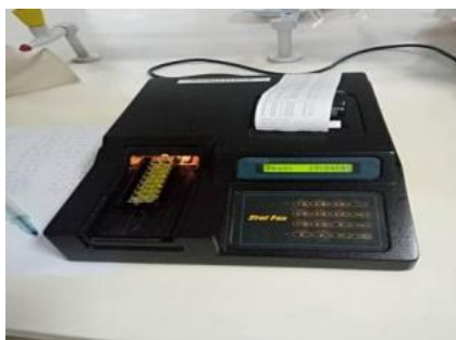
ELISA Machine for Aflatoxin Analysis. Accessories for the Preparation of Samples and Test kits
