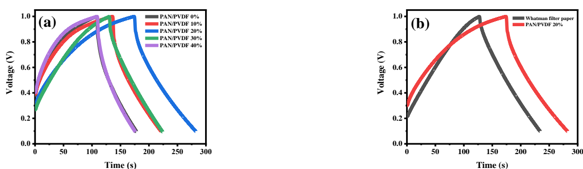
Figure 5 Supercapacitor charge-discharge: (a) PAN/PVDF nanofiber separator membrane, (b) comparison of commercial separators.
