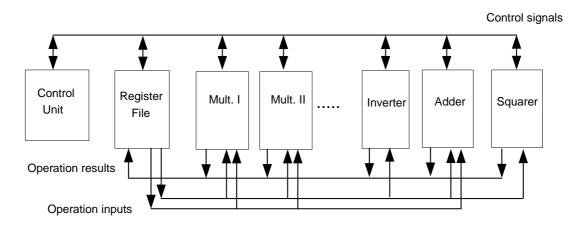
Figure 1. Crypto-processor architecture.
