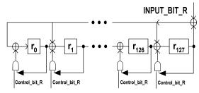
Figure7: The Implementation of Register R
