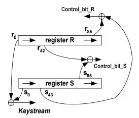
Figure5: The MICKEY-128 Block Diagram
