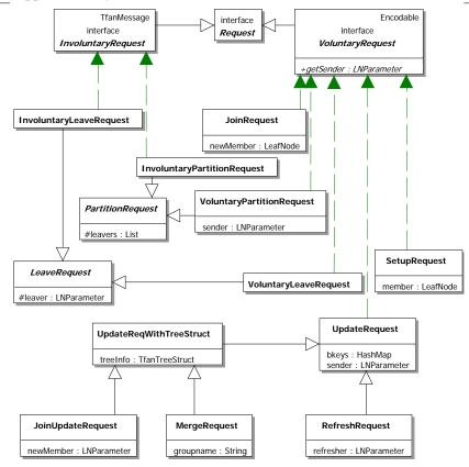
Figure 6.8.: UML diagram of request components
