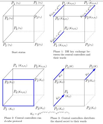
Figure 4.4.: Key exchange's process of  $2^d$  octopus (d = 2, n = 7)
