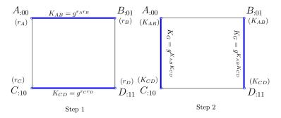
Figure 4.3.: Key exchange's process of d-cube (d = 2)
