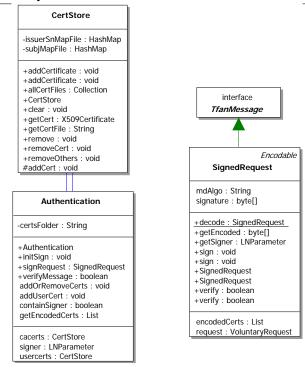
Figure 6.5.: UML diagram of components in authentication layer
