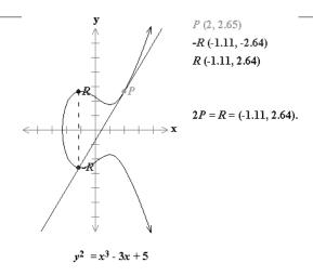
Figure 2.4.: Doubling the point P with  $y_P \neq 0$  on elliptic curve  $y^2 = x^3 - 3x + 5$
