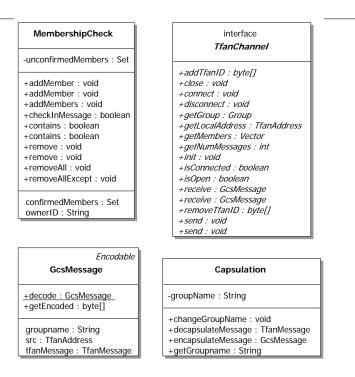
Figure 6.4.: UML diagram of components in GCS layer
