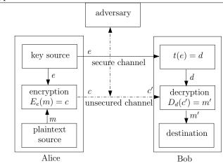
Figure 3.1.: A two-party communication using symmetric-key encryption
