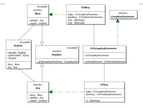
Figure 6.6.: UML diagram of key components
