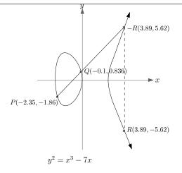
Figure 2.2.: Adding two distinct points P and Q with  $-P \neq Q$  on elliptic curve  $y^2 = x^3 - 7x$
