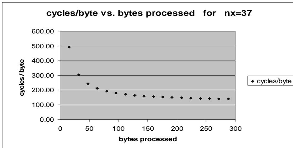
Figure 6. Cycles/byte versus bytes processed for Hermes8-128
