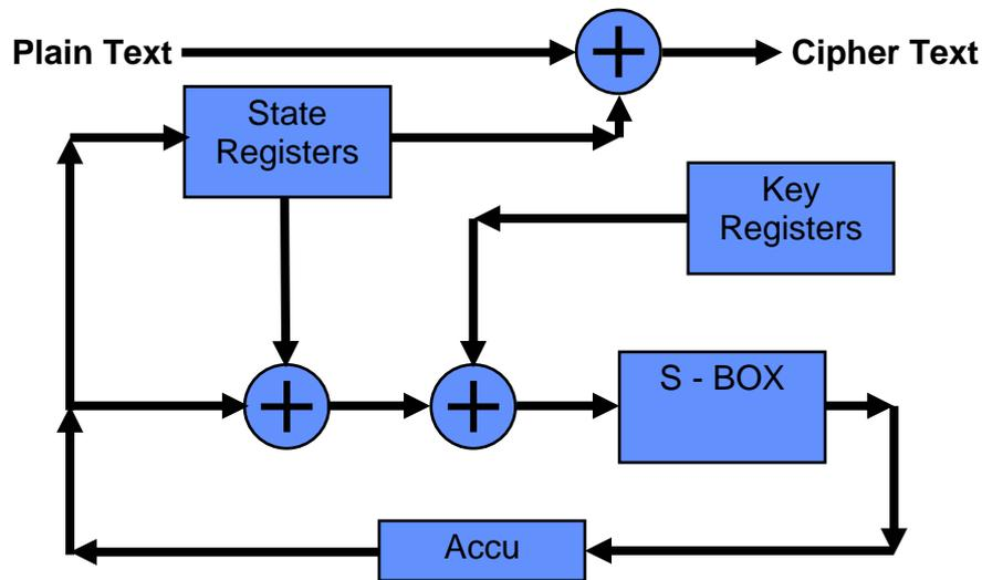
Figure 1. Principle of Hermes8 core operation round
