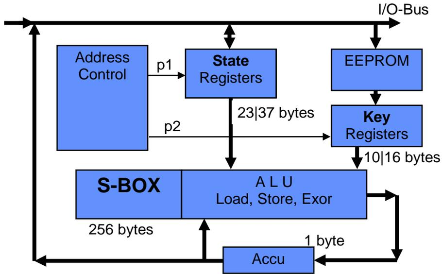
Figure 2. Byte-Architecture of Hermes8 with registers, ALU, and S-BOX
