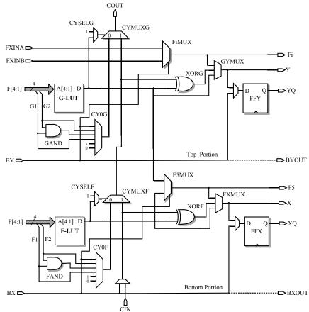
Figure 2. Simplified architecture of a Spartan-3 slice.
