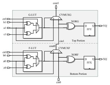
Figure 3. Three input adder architecture in one slice.
