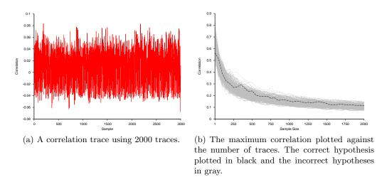
Fig. 2. Results of a DPA attack on the masked implementation demonstrating that no information leaks.
