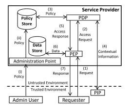
Fig. 1. The ESPOON architecture for policy enforcement in outsourced environments
