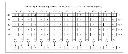
**Fig. 3.** Example of a  $16 \times 16$  - bit  $\phi$  function based on a  $5 \times 1$  - bit Boolean function  $\phi_5$ . We observe 16 and 1 cycle implementations of the same function. Note that the latter example is equivalent to "bit slicing" software implementation using rotated words.
