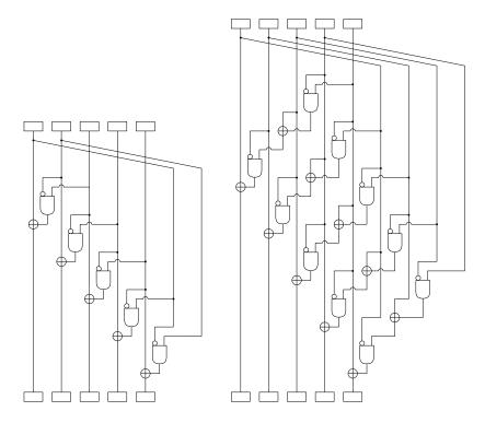
**Fig. 1.** On left, a circuit implementing KECCAK's  $5 \times 5$  - bit  $\chi$  component, which happens to be a rotation-invariant  $\phi$  function of degree 2. On right, a circuit implementing its inverse permutation,  $\chi^{-1}$ , which has Degree 3 with each output bit dependent on all input bits. Such asymmetric Boolean and circuit complexity is characteristic of  $\phi$  functions.
