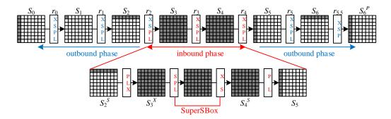
Fig. 3. Collision Attack on 6.5-Round GOST-256 Compression Function
