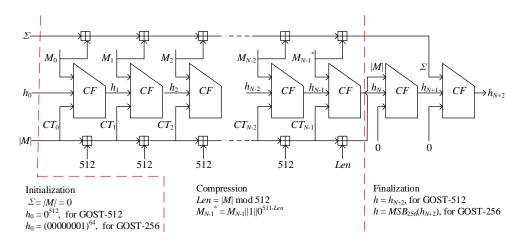
Fig. 1. Three Stages of the GOST Hash Function
