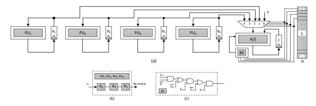
Fig. 4. BE radix-8 IMML multiplier hardware architecture
