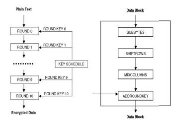
Figure 4. Iterative cipher with key schedule
