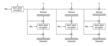
Figure 3. XTS Encryption Mode
