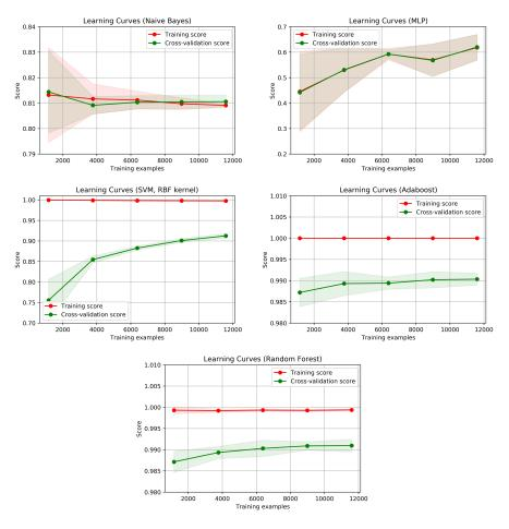
Fig. 9: Learning Curves for the classifiers in Setup 2 with 1ms granular sampling
