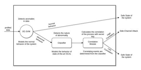
Fig. 3: Basic overview of the detection mechanism
